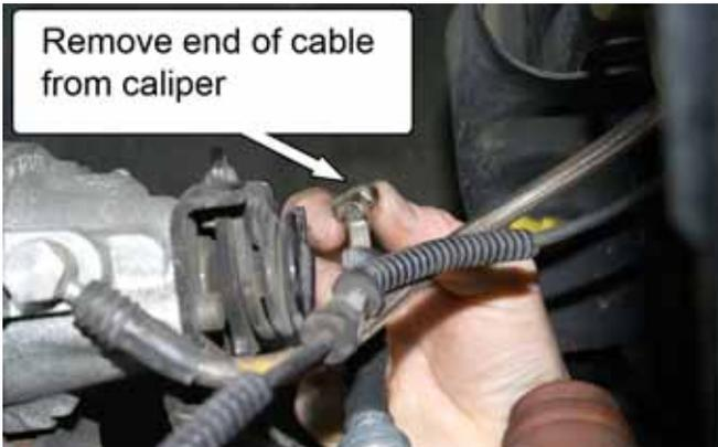
4. Slide the parking brake cable out of the slot in the OEM control arm.
