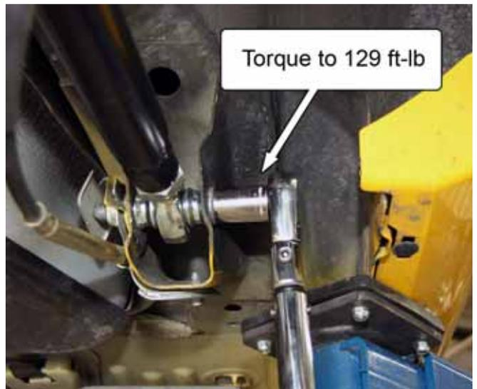
14. Route the parking brake cable under the bottom of the control arm as shown.
