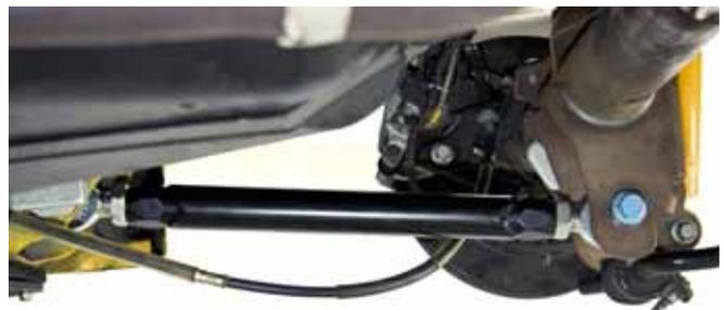
15. Reconnect the cable by slipping the end of the cable into place on the caliper, and re-installing the retainer clip removed in Step 3.
