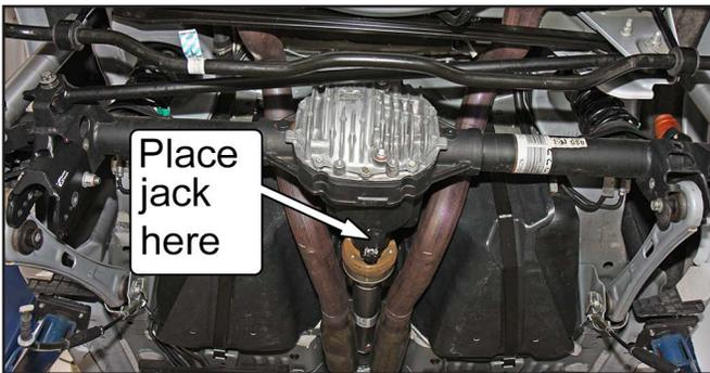
14. Remove the mounting bolt connecting the control arm to the axle housing.
