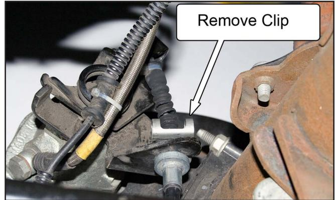
9. Pull down on the end of the parking brake cable housing and slide it rearward until it disconnects from the brake caliper.
