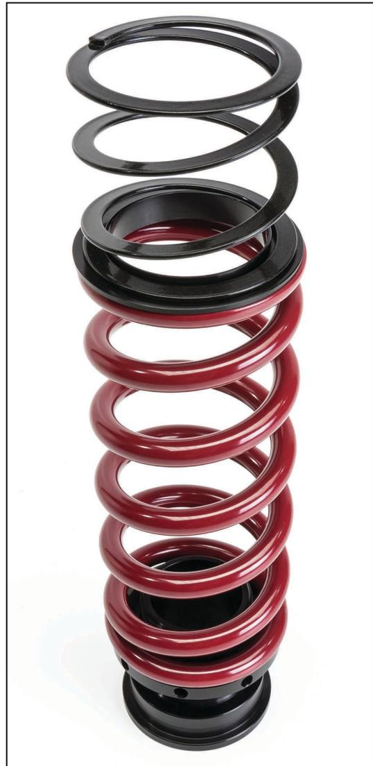
16. Take one of the spring assemblies and insert it into the spring pocket on the bottom of the passenger side frame rail. Make sure the tip of the rubber isolator, located in the pocket, gets inserted into the center of the helper spring.
