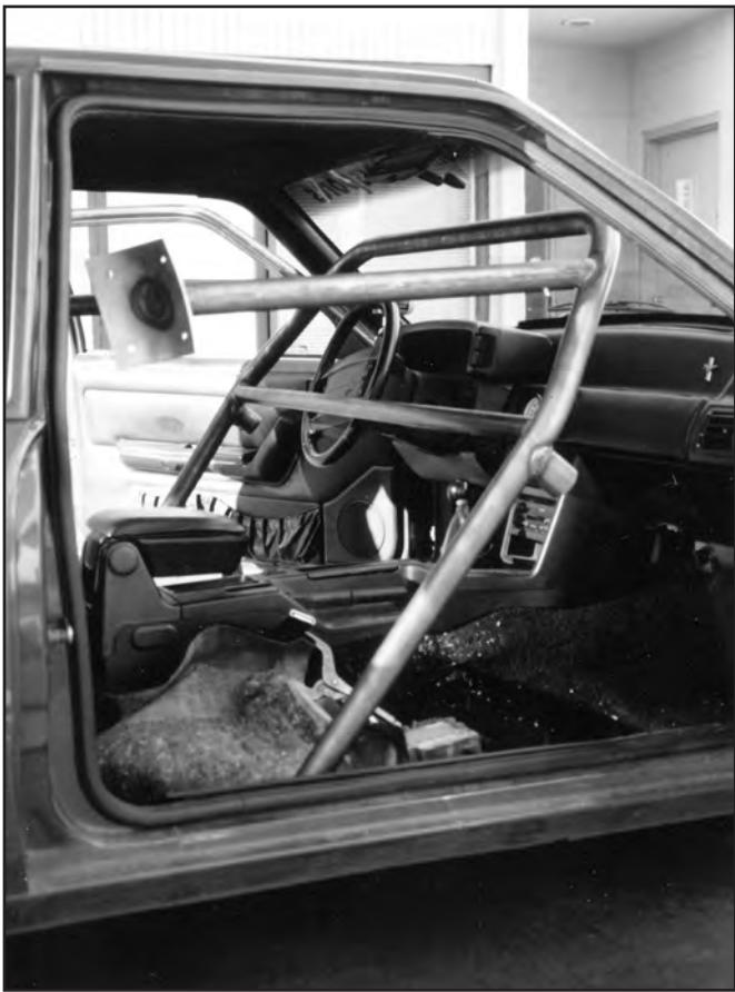
14. Slide the main hoop rearward so all mounting pads are in the correct position. The main hoop mounting pads should be centered side to side and flush with the rear seat bulkhead. *Hatchback*: The main hoop with the driver-side rear brace will set in the car as a tripod.
