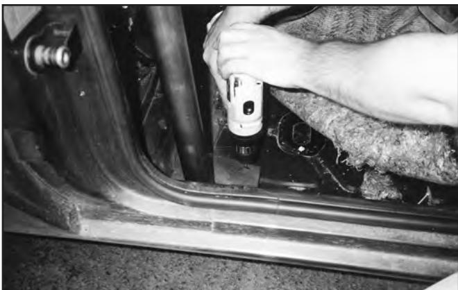
20. Place the backup plate in position and put three bolts in place, but do not tighten.
