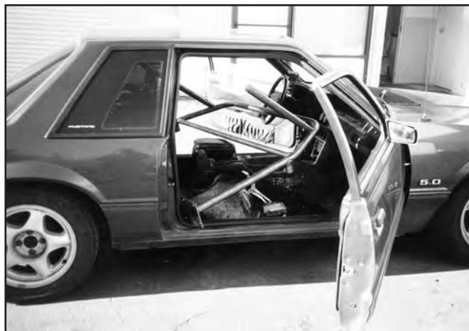
11. Tilt the main hoop upward and rearward to clear the steering wheel.
