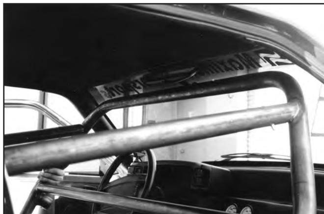
12. Pull the main hoop forward so the mounting pads are about 8–10" forward of the rear seat bulkhead.
