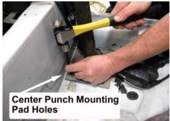
57. Put the convertible top down and slide the Main Hoop forward so that you can gain access to the center punch marks.
