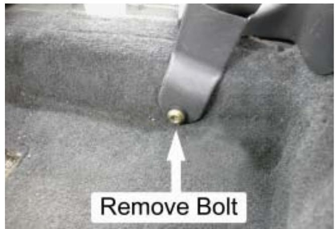
NOTE: If your vehicle has a seat belt retractor mechanism located at the inner portion of the rocker panel, you must remove its plastic cover to gain access to the mounting bolt.
