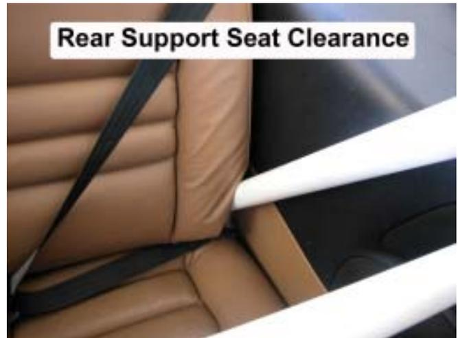
85. Once you are satisfied with the position of the Rear Supports, remove the rear seats and finish welding the Rear Supports to the Main Hoop and the Rear Support Pads.
