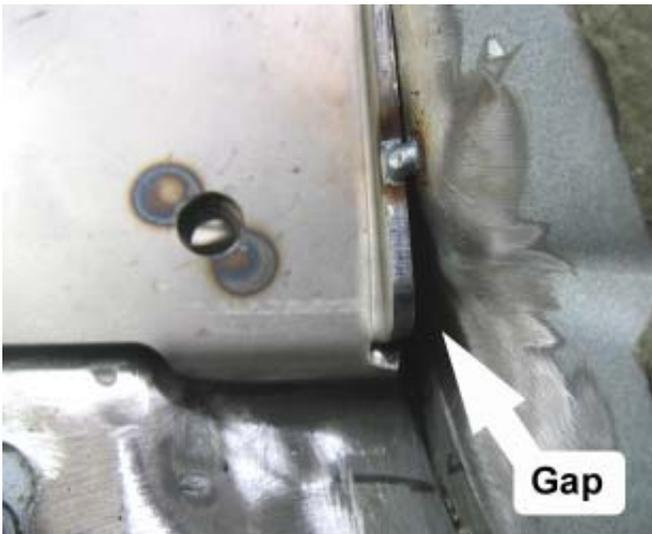
36. Using a small hammer, bend the lower portion of the flange towards the fender well until the gap is reduced by half.
