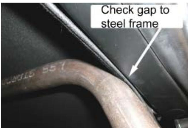
55. Double check that the Main Hoop is lined up with the marks made in Step 52.
