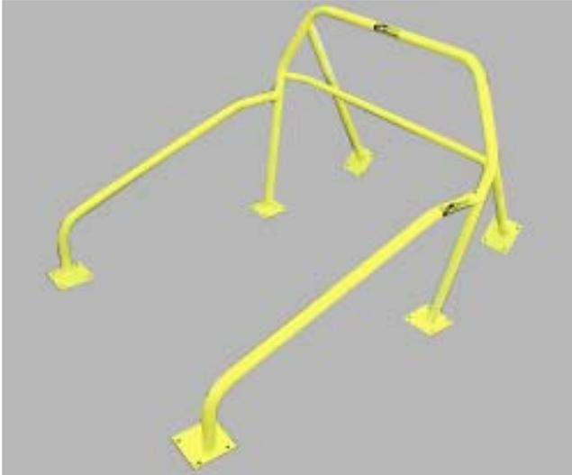
The Maximum Motorsports 6-point Drag Race Roll Bar is designed to meet the NHRA rules with proper installation. It is made from 1-3/4" x 0.134" wall DOM tubing (which exceeds the NHRA requirements of 0.118" ERW tubing). The harness mount tube is 1-1/2" x 0.134" wall DOM (NHRA minimum requirement is 1-1/4" ERW). Mounting pads and reinforcing plates are all 6" x 6" x 1/8".
