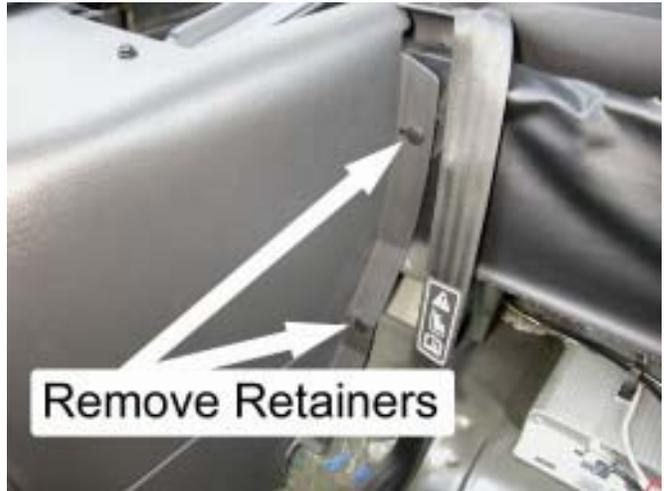
12. Begin removal of the driver and passenger rear plastic side panels by first removing the four plastic retainers holding each side panel to the vehicle. Then pull the panels away from the B-Pillar.
