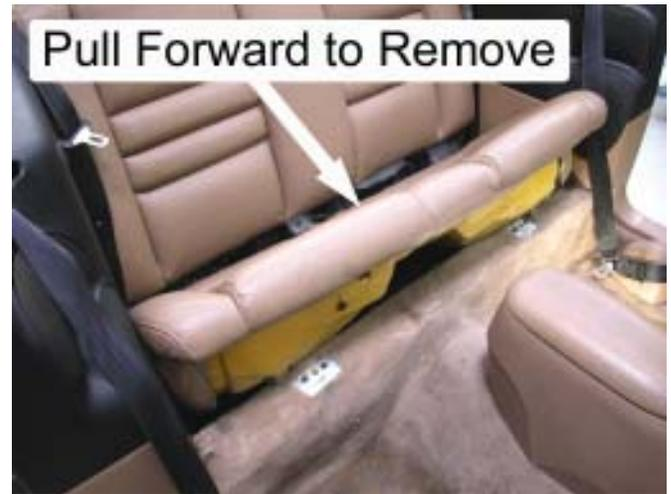
9. Remove the rear seatback from the vehicle by first removing the retaining screw holding each lower corner of the seatback to the vehicle. Then, carefully pull the seatback straight up and out of the vehicle.
