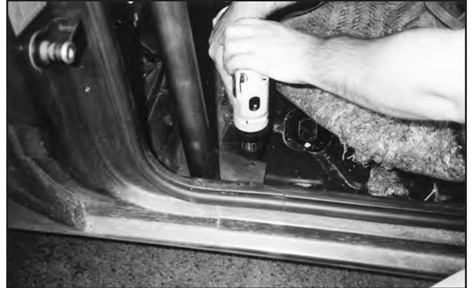
20. Place the backup plate in position and put three bolts in place, but do not tighten them yet.
