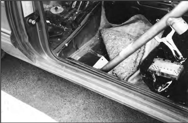
13. Keeping the main hoop mounting pads in about the same forward position, tilt the main hoop rearward so the rear brace mounting pads move toward the rear wheel well housings.
