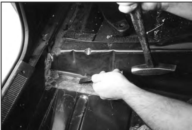
4. Remove the sound deadening on the rear inner wheel well where the rear brace mounting pads will rest.
