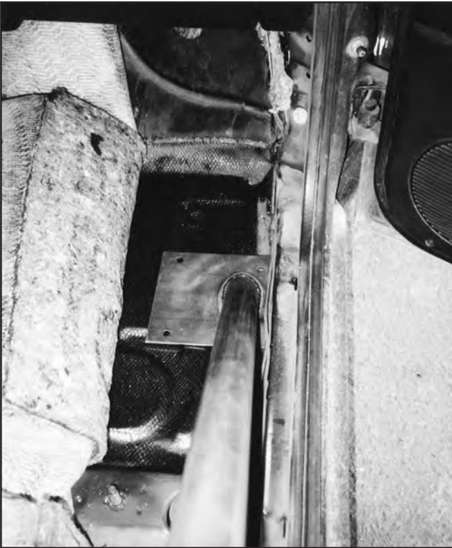
18. Close the doors and check for arm-rest clearance. The door bars may press lightly against the arm-rests.
