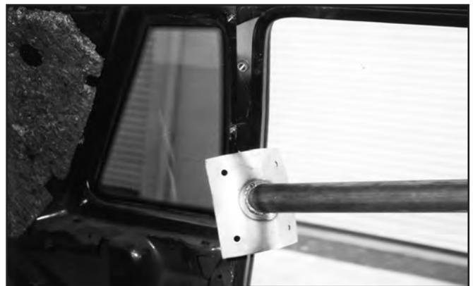
14. Slide the main hoop rearward so all mounting pads are in the correct position. The main hoop mounting pads should be centered side to side and flush with the rear seat bulkhead. *Hatchback:* The main hoop with the driver-side rear brace will set in the car as a tripod.
