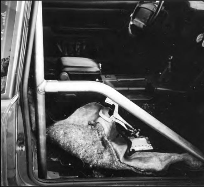
17. The door bar mounting pads should be flush with the rocker panel. *Swing-out door bars:* The edge of the mounting plate that the socket tube is closest to is the edge to place next to the rocker panel.
