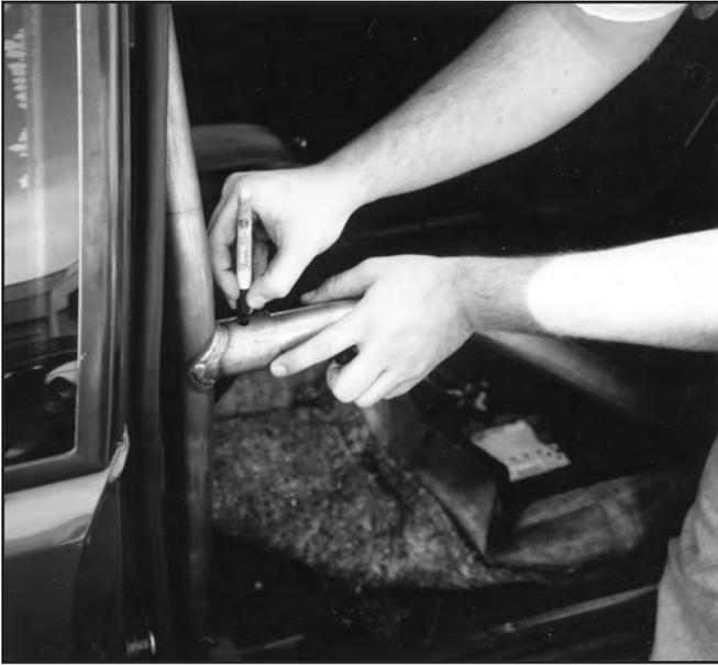
29. Place the door bars into position and insert the 2 1/2" bolts at the main hoop.
