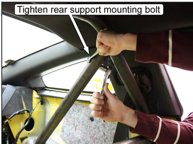
58. Remove the roll bar from the vehicle, with the rear supports firmly attached.
