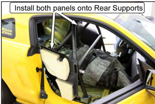
71. Lift the roll bar, along with the plastic panels, into position.
