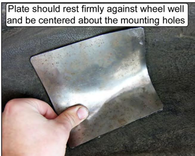
38. With the doubler plate held in position, have someone mark the location of the mounting holes from the inside of the vehicle using a center punch or marker.
