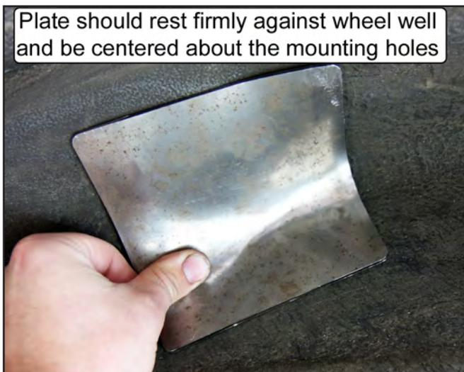
38. With the doubler plate held in position, have someone mark the location of the mounting holes from the inside of the vehicle using a center punch or marker.
