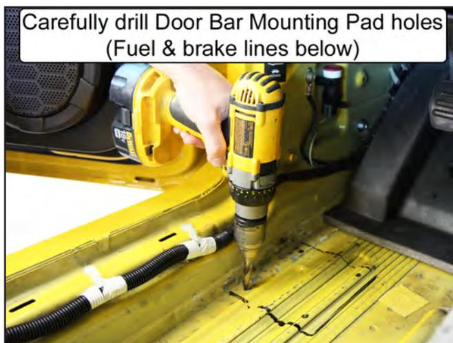
**NOTE:** There ARE fuel and brake lines directly beneath the driver-side door bar mounting pad. Place the door bar doubler plate between the underside of the floor pan and the lines as a shield when drilling to prevent punctures.
