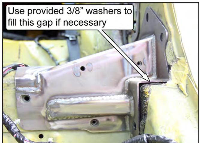
20. Check the gap between the bracket and the vehicle at H8. Use the provided 3/8" G8 washers to close the gap to 1/8" or less. When satisfied, insert one of the factory mounting bolts into the hole to prevent the washers from being dislodged.
