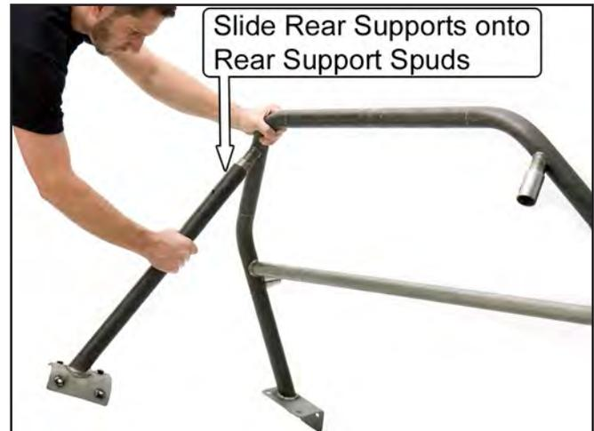
26. Place the roll bar into the vehicle by tilting the hoop forward and passing it through the passenger-side door. Once the roll bar is in the vehicle, tilt it rearward and place it onto the MM support brackets and the rear support mounting pads on the inner corner of each rear wheel well.
