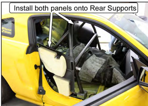
71. Lift the roll bar, along with the plastic panels, into position.
