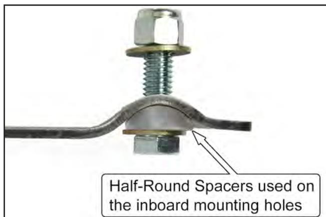
87. Torque the entire door bar mounting hardware to 33 lb-ft.
