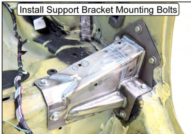
22. Using a wrench, tighten (but do not torque) all bolts in numerical order from H1 to H9 so the bracket can be properly seated on the vehicle.
