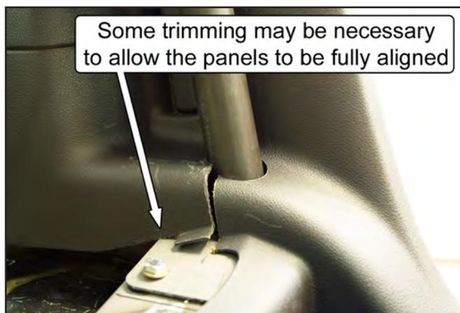
78. Reinstall the safety belts to the rocker panels and torque the T-47 Torx bolts to 30 lb-ft (40Nm).
