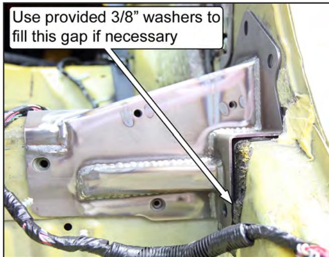
21. Install the remaining mounting bolts into the support bracket and tighten them by hand. Take note that H6 and H7 use the larger, 15mm hex head bolts.
