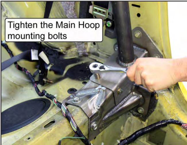
33. With both rear support mounting pads in their proper position (resting firmly against each rear wheel well), tighten the two bolts holding the rear supports to the main hoop so the rear supports CANNOT move.
