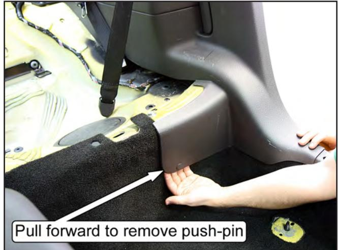
11. Remove the rear quarter panels. There are three push-pin retainers on each panel; one is located at the front of the seat bulkhead and two are at the rear seat backrest. Carefully pull the rear half of the panels inwards to disengage the snap-in retainers located below the quarter window, and then pull the panels forward.
