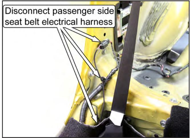
15. Relocate the wiring harness in the area adjacent to each B-pillar. Unfasten the harness retaining clips from the vehicle and pull the harness inboard to clear the factory support brackets. If necessary, you can get more slack by disconnecting the harness where it plugs into each of the seatbelt retractors.
