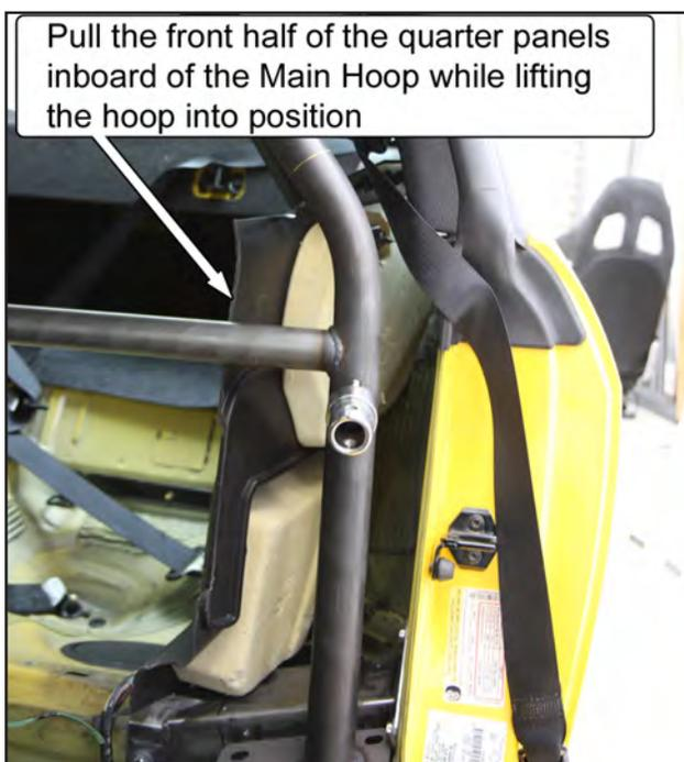
72. Reinstall all the mounting hardware for the main hoop and rear supports before tightening any of the bolts. The main hoop uses 3/8"-16 x 1"-long bolts with a 3/8" G8 washer under the bolt head. The rear supports use 3/8"-16 x 3/4"-long bolts and 3/8" G8 washers beneath the bolt heads.
