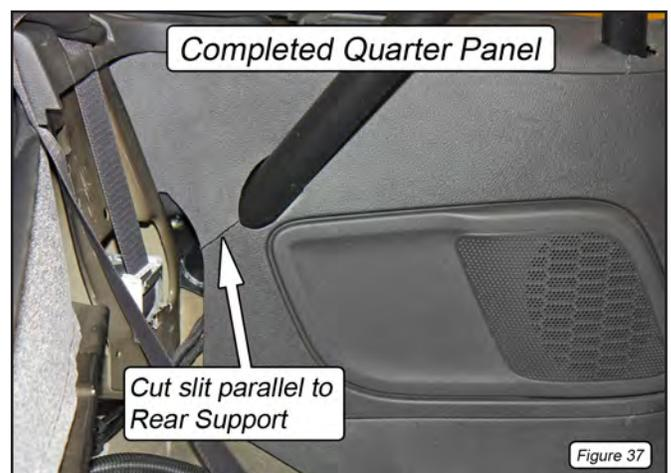
55. Repeat Steps 46-54 for the passenger side of the vehicle with the driver-side rear support installed and the passenger-side rear support removed.
