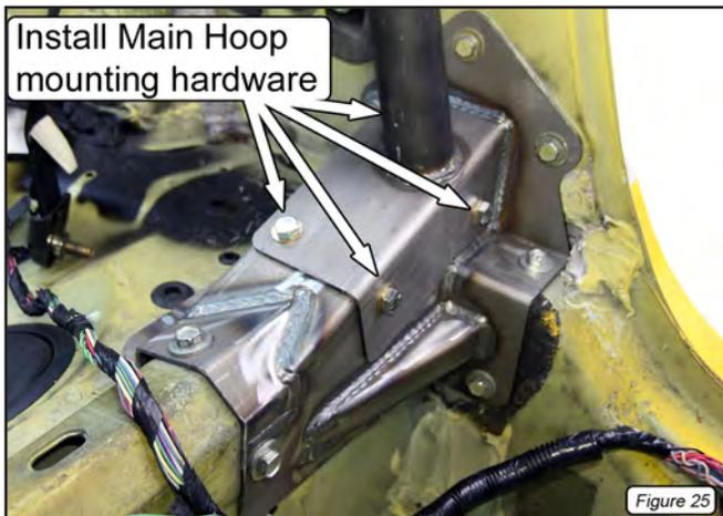
32. Temporarily tighten the bolts that secure the hoop to the MM support brackets (Figure 26).
