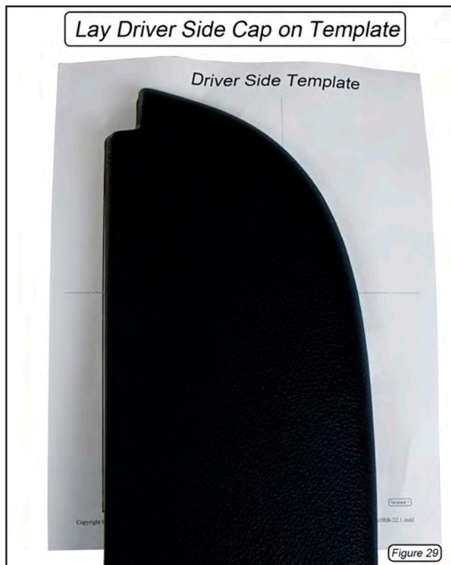
42. Use a ruler to extend the horizontal and vertical lines from the template across the cap until they cross. The point at which they cross is the center of the roll bar tube (Figure 30).
