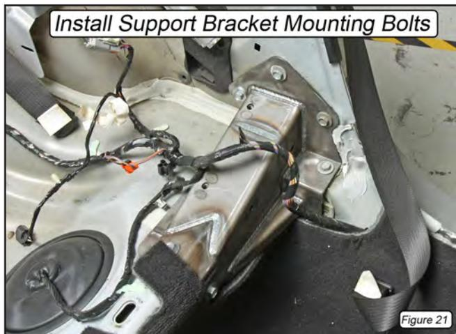
25. Using a wrench, tighten (but do not torque) all of the bolts in numerical order from H1 to H9 so the bracket can be properly seated against the vehicle.
