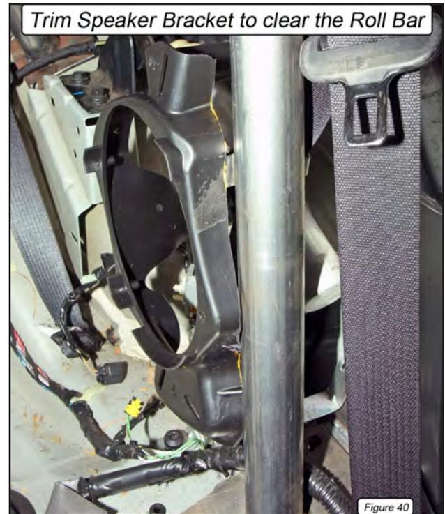
76. Once satisfied, place the speaker bracket into position and drill a 1/8" hole through the bracket, in line with the hole in the L-bracket welded to the vertical portion of the Main Hoop (Figure 41).
