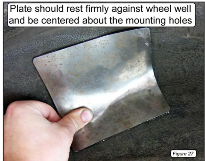
38. With the doubler plate held in position, have someone mark the location of the mounting holes from the inside of the vehicle using a center punch or marker. There must be a minimum of ¼" between the edge of the doubler plate and the edge of each mounting hole (Figure 28).
