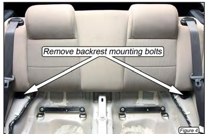
7. Gently unclip the convertible top from the backrest and remove the backrest by lifting it vertically.
