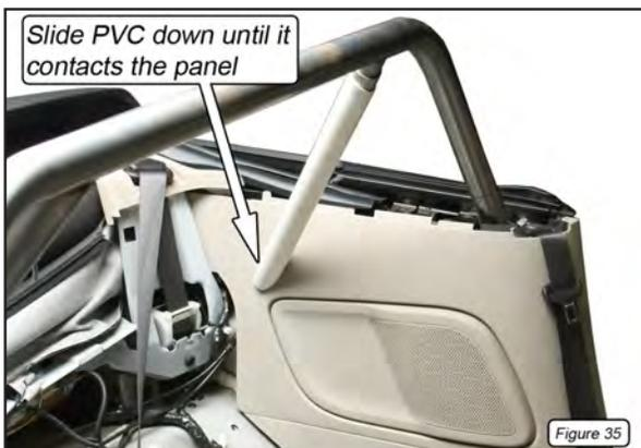
50. Use a marker to trace around the PVC template, the location where the rear support will pass through the plastic panel.
