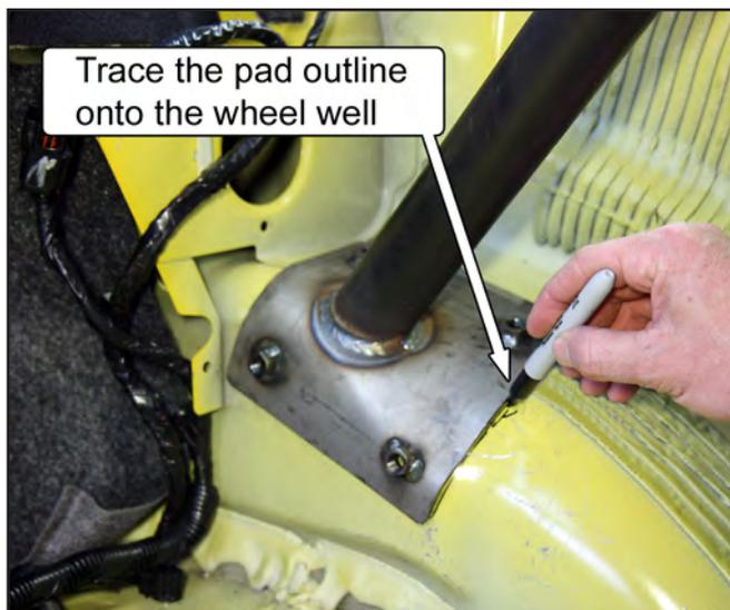
28. Remove the sound-deadening material within the outline using a chisel or other scraping device. Then reinstall the roll bar into the vehicle.
