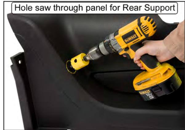
54. Cut a vertical line from the bottom of the plastic panel up to the rearward edge of the hole. This will allow the panel to be slid onto the rear support during installation. Use sandpaper or a file to remove any burrs from the edge of the plastic panel.
