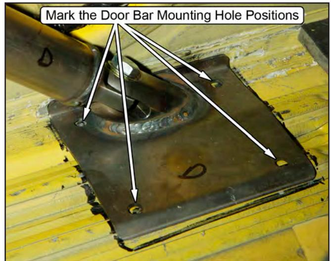
36. Remove the roll bar from the vehicle and drill the four holes marked on each wheel well out to a 7/16" diameter. Use ~1/8" diameter pilot drill to start the holes.
