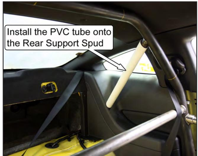
51. Set the roll bar back in its mounting position and slide the PVC tube down until it contacts the plastic quarter panel. Rotate the PVC tube so the end is parallel to the face of the panel.
