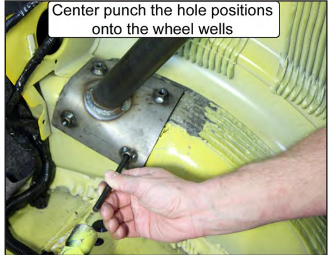
35. Mark the position of the four mounting holes in each door bar mounting pad onto the floor pan using a center punch.
