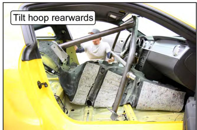
27. Trace an outline of the rear support mounting pads onto the driver- and passenger-side wheel wells, and then remove the roll bar from the vehicle.
