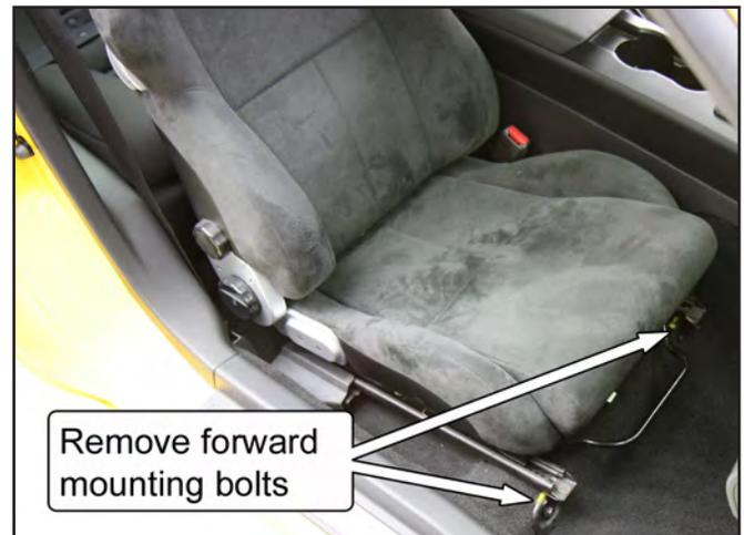
4. Tip the seat back to disconnect the wiring harness connectors for the air bag module and seat. Carefully pull the seats out of the car and place aside.
