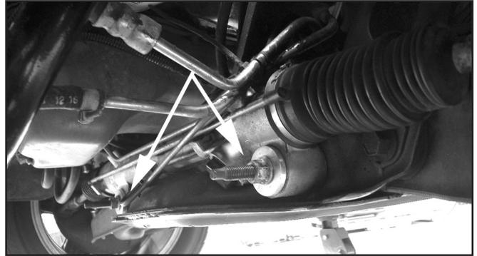
6. Pull the steering rack forward just far enough to allow the steering shaft to slip off of the steering rack input shaft. It is not necessary to disconnect the power steering system hoses.
