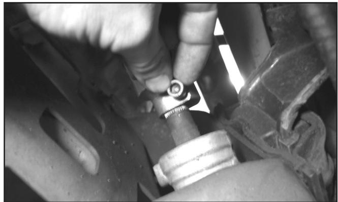
*NOTE: Make sure the Lower U-joint pinch bolt is inserted through the unthreaded side of the U-joint first and then into the threaded side. This will allow the U-joint to clamp onto the threaded shaft when the bolt is tightened.*
