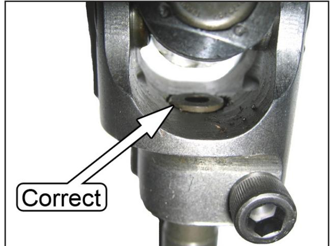
28. Reconnect the lower U-joint to the steering rack input shaft by extending the telescoping steering shaft enough to slip the splines together. If loosened, torque the steering rack mounting bolts to 40 ft-lbs.
