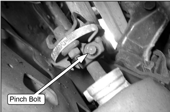
*NOTE: Most aftermarket steering shafts are secured to the input shaft with a setscrew and jam nut. Loosen the jam nut, and back out the setscrew.*
