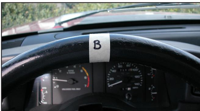
21. Divide the number of turns required to go from full lock to full lock in Step 19, by 2.
