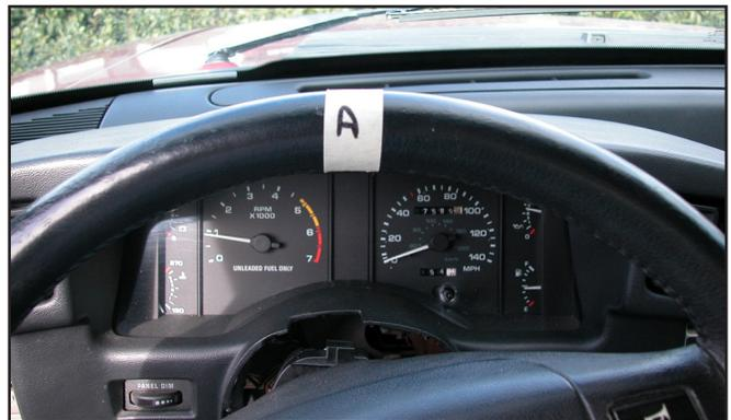
19. Rotate the steering wheel counter-clockwise until full lock is reached. For future reference (in Step 20), count the number of turns required to turn the steering wheel from full lock to full lock.
