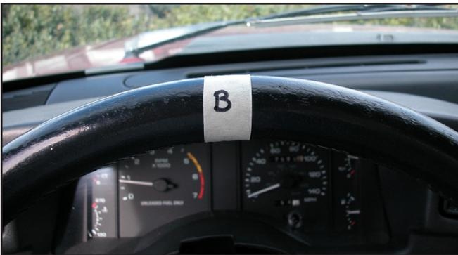
25. Divide the number of turns required to go from full lock to full lock in Step 23, by 2.
