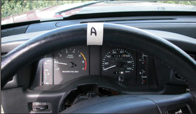
23. Rotate the steering wheel counter-clockwise until full lock is reached. For future reference (in Step 24), count the number of turns required to turn the steering wheel from full lock to full lock.
