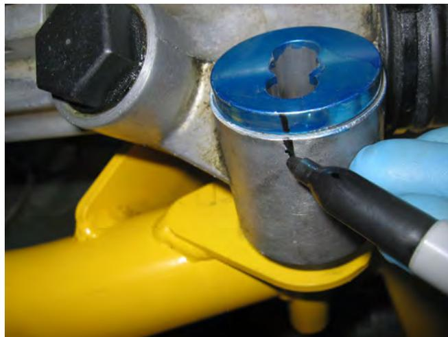
9. Place the female half of the rear Spherical Rack Bushings into the rear of the rack mounting holes. The concave portion of the bushings should face rearward in the vehicle. Orient the three holes so that they match the orientation of the holes in the front aluminum rack bushings.
