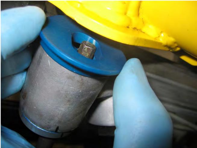
13. Fully insert the bolt into the k-member rack mounting holes. Make sure the bolt is passing through the correct offset-holes in the rack bushings.
