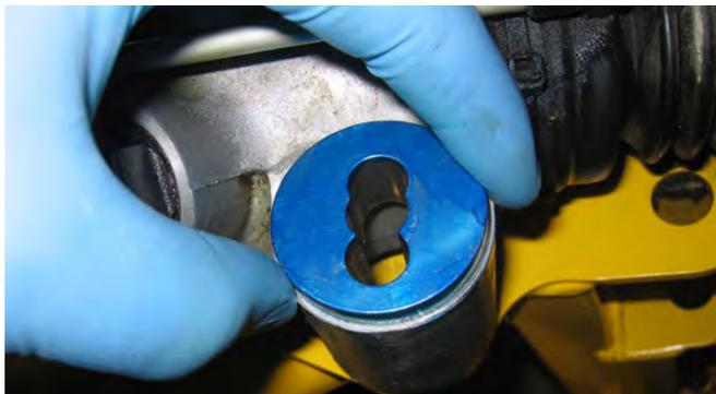
8. Using a marker, or other marking device, make an indicator line across the edges of the steering rack bushings and the steering rack housing. These lines can be used to determine if the rack bushings have rotated out of their position during later steps.
