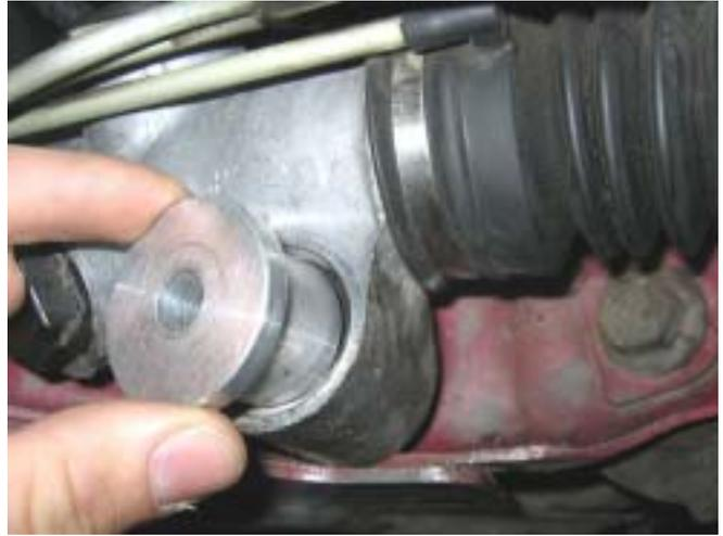
14. Slide the rack mounting bolts in from the rear of the k-member far enough so that they protrude about an inch past the front steering rack mounting face of the k-member. Make sure the sleeves are resting against the rear of the k-member. The front of the sleeve must be in the hole at the front of the k-member, and also should not protrude past the forward face of the k-member.
