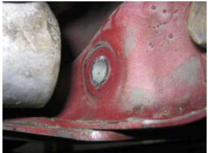
10. Place the rear half of the MM aluminum rack bushings (with the machined concave mounting face) in the rearward side of the steering rack mounting holes.
