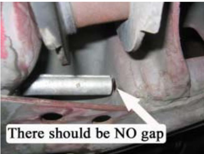
7. Remove the steering rack mounting sleeves from the k-member. Mark each sleeve as to which side of the vehicle they were removed from.
