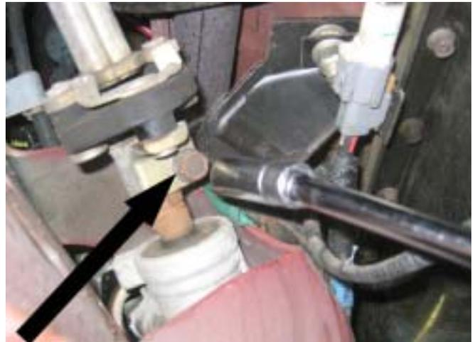
3. Remove the two nuts and washers holding the steering rack to the k-member.
