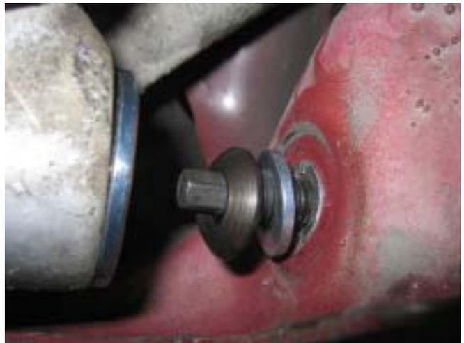
17. Place the steering rack back into position, using the rack mounting bolts as your guide. Be sure to connect the steering rack input shaft to the steering shaft at this time.
