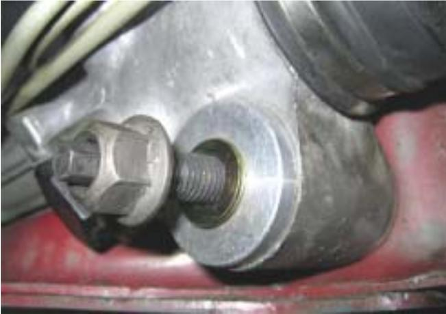
19. Reinstall the nuts on the steering rack mounting bolts, and torque to 45 ft-lbs.
