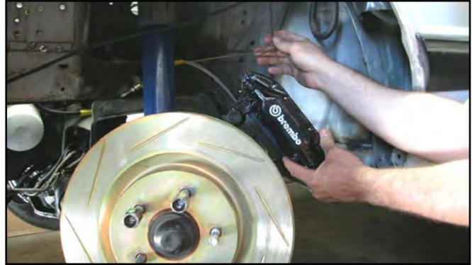
4. Remove the front brake rotor.
