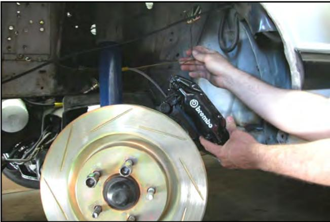
6. Remove the front brake rotor.
