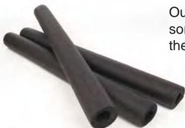
Our standard race padding is a black, high-density, fire-resistant foam that progressively absorbs shock. The offset ID allows easy installation with the thicker side of the padding toward the driver. Fits 1-3/4" diameter tube.
