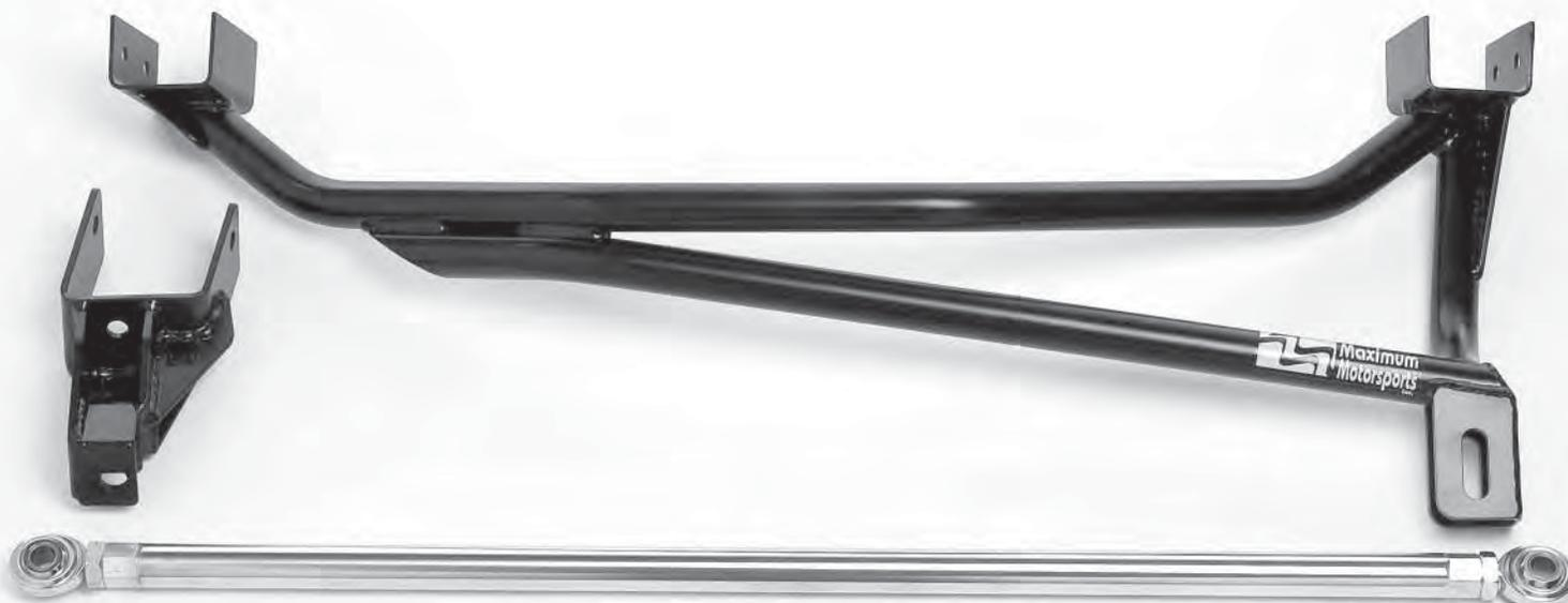
Dramatically improve your Mustang's handling by eliminating the unstable and unpredictable behavior caused by rear-steer. Installing a Maximum Motorsports Panhard Bar halts the unwanted axle movement that causes the rear of the car to steer itself. This easy-to-bolt-on part is mandatory for a Mustang to achieve truly great handling!
