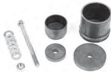
This tool from MM makes it much easier to change the stock rear upper control arm bushings at the differential (Part E4SZ-5A bushings). The bushings are a press fit in the differential housing, and are difficult to access. They're especially difficult to change if you're trying to do so without removing the rear axle assembly from your car. MM's unique tool makes this tough job much easier and faster.
