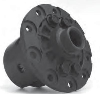
During braking there's little or no torque being conveyed to the differential, so there's little or no torque difference between the two rear tires. Therefore, the Torsen differential will not support any appreciable torque "wind-up" between the two rear tires during braking. For that reason the Torsen differential does not interfere with the functioning of anti-lock brake systems.
