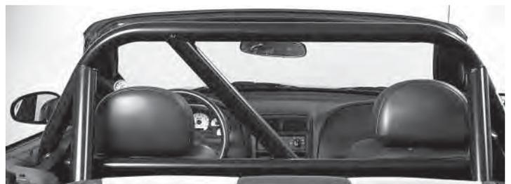
MM Roll Bar with diagonal brace installed
