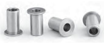
The Maximum Motorsports Stainless Steel Brake Caliper Sleeves replace the factory rubber bushings. Rubber lets the calipers move during braking, preventing the pad from contacting the rotor surface squarely. This movement reduces your brakes' effectiveness and leads to tapered pad wear. These caliper sleeves also fit the 73mm SVO calipers.
