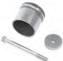
This tool easily removes the stock rubber IRS rear differential bushing from its mounting bracket.
