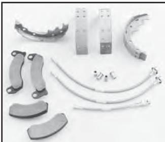
Reduces stopping distances by 12-15 percent! This upgrade package includes Hawk brake pads (HB-263 HPS), MM High-Performance Rear Shoes, MM Stainless Steel Caliper Sleeves, and MM Stainless Steel Brake Hoses (3-hose kit). The complete MM Brake Upgrade Package produced an average stopping distance of 114 ft from 60 mph, with the shortest distance at 98 ft (*Mustang Monthly*, Sept. 1993). For more information, also see the article in *Super Ford*, July 1994.
