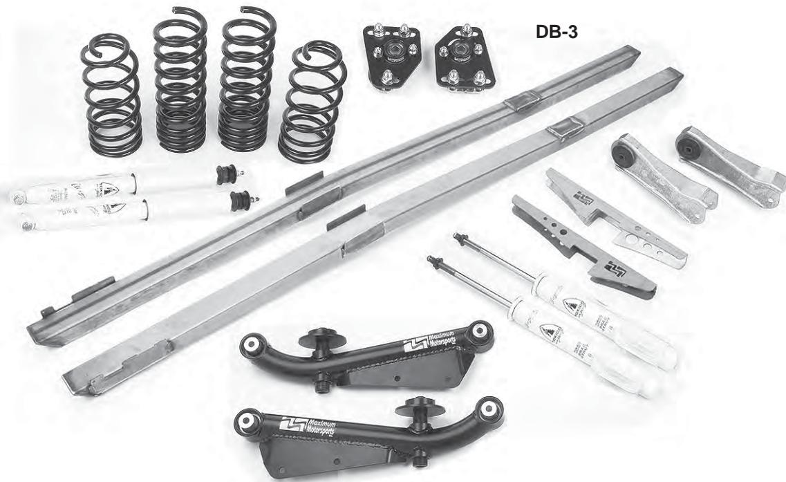
This Grip Box was designed with a minimalist approach to modifications, and is intended for the occasional drag racer on a budget. It will improve launch consistency and increase durability with just the right combination of parts.
