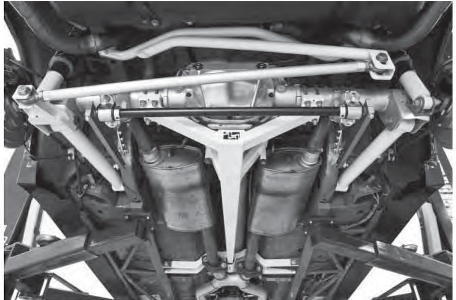
MM Panhard Bar, shown installed along with other Maximum Motorsports parts.
