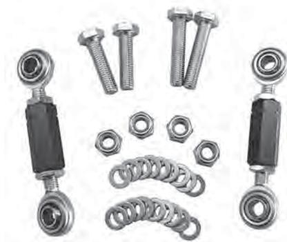
The MM endlinks allow adjustment to eliminate the swaybar preload that occurs when one of the endlinks is not exactly the correct length for a particular installation. The swaybar twists and becomes preloaded if the endlink length is off by even a very small amount. The preload will alter the car's corner weights, which in turn causes asymmetrical handling characteristics.
