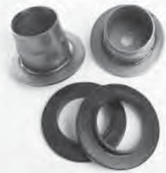
This adapter allows fitting a standard 2.5"-diameter coil-over spring in place of the standard rear spring. Welds to the chassis in the center of the stock upper spring perch. Includes urethane upper spring isolators for 2.5"-diameter springs.
