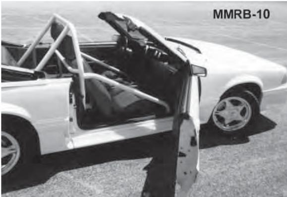
Increase both your safety and your Mustang's chassis rigidity with a Maximum Motorsports Roll Bar. We offer 6-point roll bars for drag racing (meets NHRA and NMRA requirements) and 4-point roll bars for road racing and street use. Several options are available: diagonal braces; fixed or removable harness mount tubes; and low-slung, fixed, or removable swing-out door bars.
