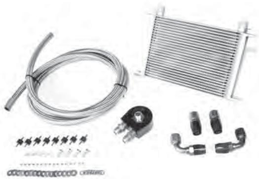
A must-have for any high-power engine, this system keeps engine oil temperatures in check at the track and on the street. At the heart of this kit is a 25-row aluminum liquid-to-air heat exchanger. Its all-aluminum plate construction makes this one of the best coolers available, greatly outperforming “tube and fin”-style units. PTFE-lined stainless steel braided hoses with -10AN fittings, aluminum mounting brackets, and vibration-insulating standoffs round out this complete package.
