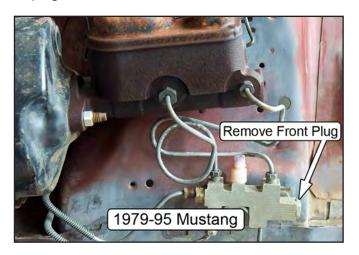
NOTE: Be careful while loosening the plug. There is a spring pressing against the backside that will fly out.
