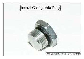
Install the MM Brake Proportioning Valve Plug in your stock brake proportioning valve and tighten to 21 lb-ft.
