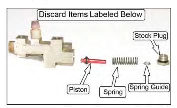
NOTE: We highly recommend using a Q-tip and brake cleaner to remove any loose debris out of the bore of the stock proportioning valve.
