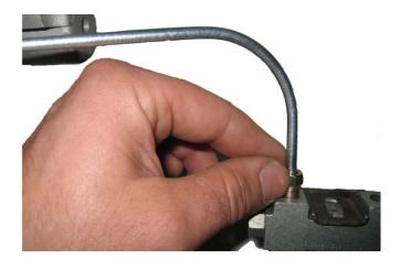
6. Thread the M12-1.0 *bubble flare* end of the supplied 1/4" brake hard line into the forward port of the stock master cylinder. Position the free end of the brake hard line above the stock proportioning valve.
