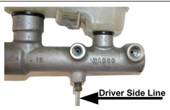
4. Thread the M10-1.0 *bubble flare* end of the supplied 3/16" brake hard line into the rear, side port of the stock master cylinder. Position the free end of the brake hard line above the stock proportioning valve.
