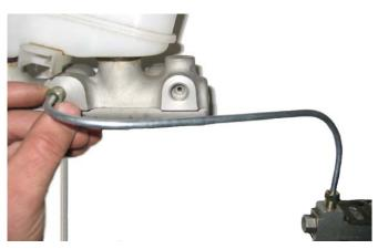
NOTE: The metric "bubble flare" can be differentiated from the standard "inverted flare" by a flare that extends past the threaded end of the fitting.
