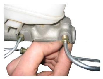
6. Thread the free end of the brake hard line into the front port of the stock proportioning valve.
