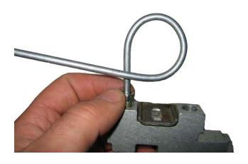
Thread the M10-1.0 bubble flare end of the "Forward Port" labeled brake hard line into the front port of the master cylinder. Position the free end of the hard line above the stock proportioning valve.
