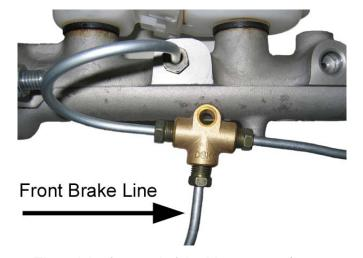
4. Thread the free end of the M10-1.0 to 3/8-24 brake hard line, connected to the remaining port on the Tee fitting, into the rear port of the stock proportioning valve.
