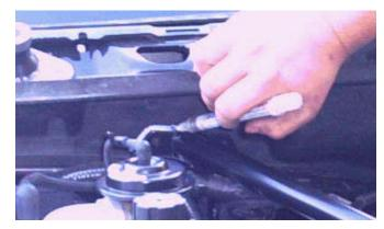
7. Remove the Strut Tower Brace.
