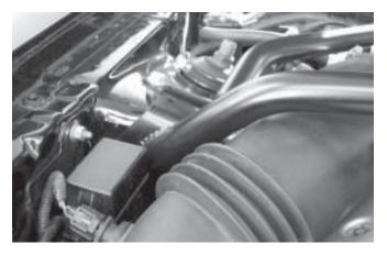
Be sure that both firewall mounts of the brace are held down against the firewall pinchweld. Mark the position of the firewall mounts on the plastic firewall cover. The cover will be trimmed in Step 9.
