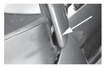
Remove the plastic cowl cover at the base of the windshield. It is held on with clips. Remove it by gently prying it upwards. When it is loose, disconnect the hose to the windshield washer nozzles (pointed to below).
