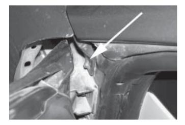
18. DO NOT remove the applique. Gently move it away just enough to open a small gap for removal of the plastic cowl at the base of the windshield.
