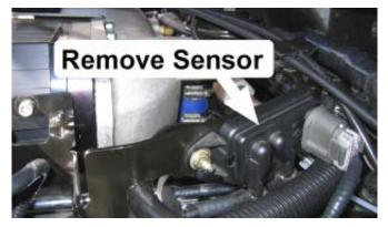
8. Push the studs out of the sheet metal bracket that were used to secure the pressure sensor. Place a small socket over the head of the stud and use a large pair of pliers to push the stud into the socket.
