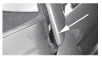
26. Remove the plastic cowl cover at the base of the windshield. It is held on with clips. Remove it by gently prying it upwards. When it is loose, disconnect the hose to the windshield washer nozzles (pointed to, below).
