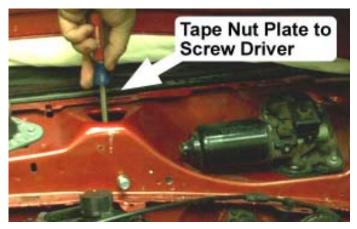
40. Install the #8 sheet metal screw into the small hole in the nut plates. Remove the 5/16-18 bolts.
