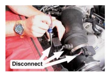
7. Unbolt the pressure sensor located on the driver side of the supercharger and remove the two vacuum lines and electrical connecter that are attached to it. The pressure sensor needs to be bolted on the opposite side of the mounting bracket to provide clearance for the strut tower brace.
