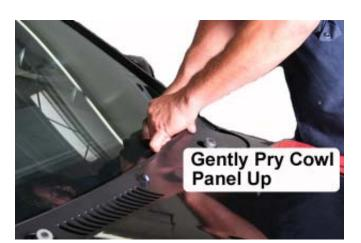
*Tip:* Remove the hood or hold it upright by using a rope or strap to tie the hood to the steering wheel.
