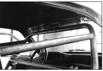
12. Pull the main hoop forward so the mounting pads are about 8–10" forward of the rear seat bulkhead.
