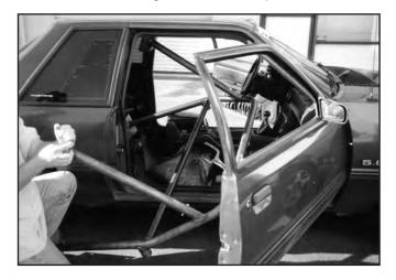
Maneuver the driver side of the main hoop up and over the center console, keeping the rear-mounting pad behind the center console.
