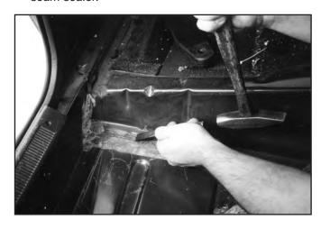
Remove the sound deadening on the rear inner wheel well where the rear brace mounting pads will rest.
