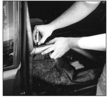
29. Place the door bars into position and insert the two  $\frac{1}{2}$ " bolts at the main hoop.
