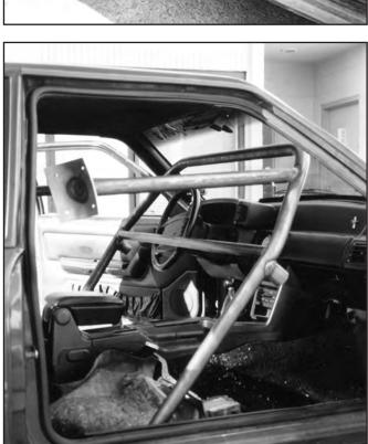
13. Keeping the main hoop mounting pads in about the same forward position, tilt the main hoop rearward so the rear brace mounting pads move toward the rear wheel well housings.
