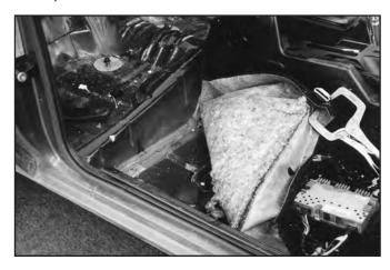
3. Remove excess body seam sealer in the corner where the main hoop mounting pads will rest on the floor pan.
