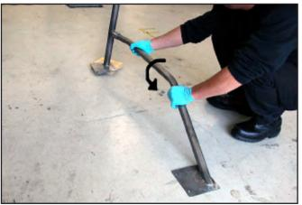
17. The door bar mounting pads should be flush with the rocker panel. *Swing-out door bars:* The edge of the mounting plate that the socket tube is closest to is the edge to place next to the rocker panel.
