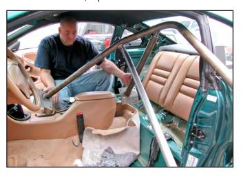
47. Keep the roll bar as low to the ground as possible in order to keep adequate clearance on the upper door frame.
