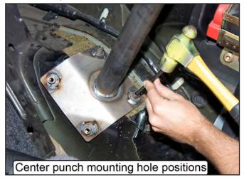
29. Move the main hoop forward and drill the four holes marked on each wheel well out to a 7/16" diameter. Use 1/8" diameter pilot drill to start the holes.
