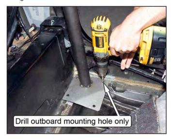
26. Drill through the forwardmost, outboard mounting hole on the passenger-side main hoop mounting plate using a 3/8" drill bit. Place one of the provided 3/8-16 x 1"-long bolts into the drilled hole.
