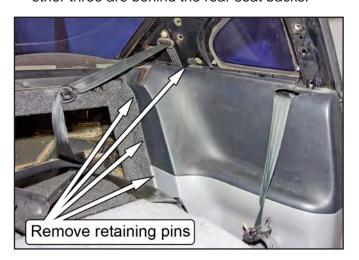
Remove the lower plastic quarter panels by pulling forward on the B-pillar edge. Once the panels unsnap, angle them out and over the rear seat bulkhead.
