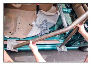
46. Continue to pull the roll bar out the door. Make sure the main hoop mounting pads clear the center console, if present.
