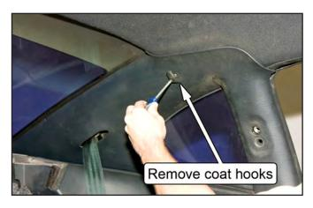
Remove the upper plastic quarter panels. They snap into place using retaining clips located on the backside of the panel. Remove the panel by pulling inboard on the upper B-pillar edge until you hear it unsnap. Then, gently pull on the lower B-pillar edge of the panel until it comes loose.
