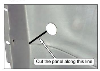
39. Continue the cut along the horizontal seam line, all the way to the rear of the panel. This will allow the panel to be slid onto the rear support during installation. Use sandpaper or a file to remove any burrs from the edge of the plastic panel.
