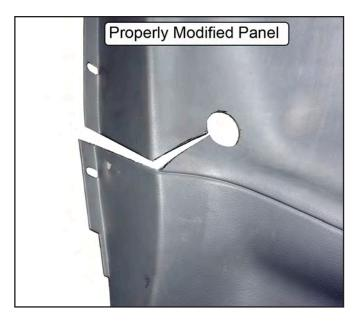
**NOTE:** 1994-98 vehicles use a less flexible plastic for the quarter panels that can't be spread apart. They require removal of a section of the panel to allow installation onto the rear supports. Remove a section of the panels as shown below.
