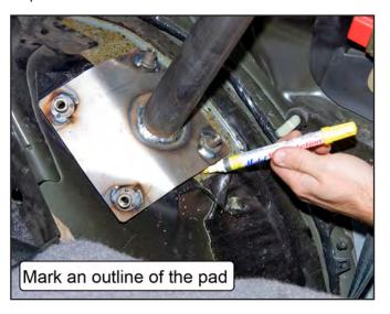
24. Move the main hoop forward and chisel away the sound insulation within the marked area on each rear wheel well. The rear mounting plates must rest directly against the metal of the wheel well.
