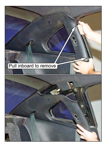
10. With the rear seats folded down, extend the rear seatbelts so that the panels can be placed in the trunk area, out of the way.
