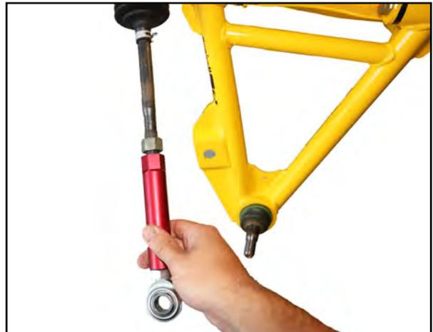
17. Insert the tapered bumpsteer stud into the spindle, and torque it to 65 ft-lb using the supplied new 1/2" nylock nut.
