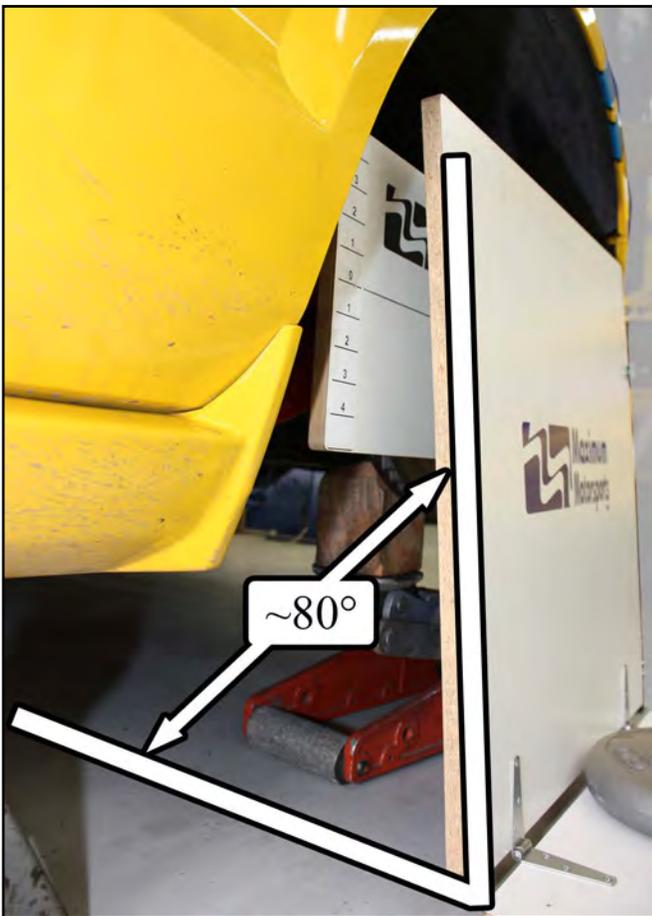
28. The dial indicator and the fixed pointer must be attached to the bumpsteer gauge at this point. When viewing the gauge from the side of the vehicle, attach the dial indicator to the rearward edge of the bumpsteer gauge and attach the fixed pointer to the forward edge of the bumpsteer gauge by hand tightening the clamp bolts. The pointers should be facing the reference plate.
