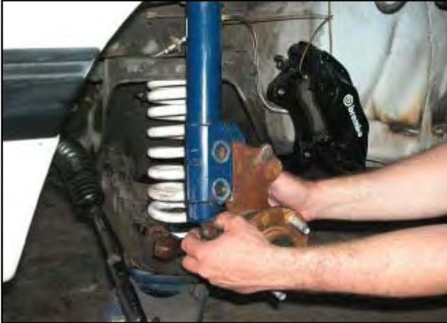
17. Remove the upper strut mounting nut. When the threads on the nut are past the nylock insert, hold the strut housing with your other hand so the strut assembly does not fall. Remove the strut from the car.
