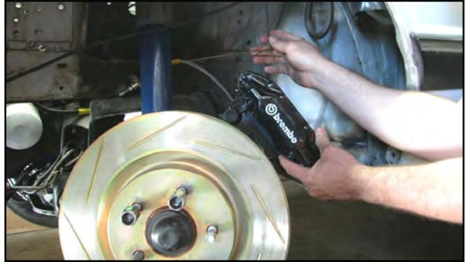
4. Remove the front brake rotor.
