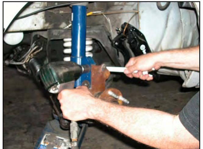
9. Remove the lower nylock nut from the Tapered Stud and remove the MM Adjustable Tie-Rod End from the steering arm.
