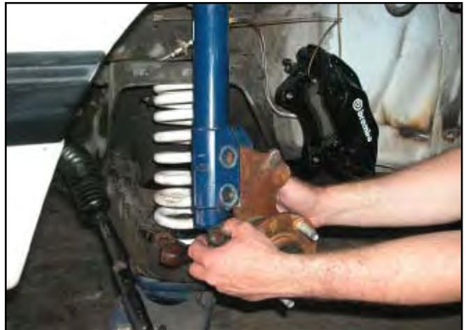
13. Carefully lower the floor jack until the front spring becomes unseated from the upper spring perch. Remove the spring from the control arm.
