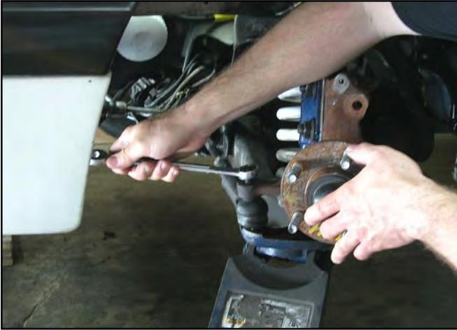
7. Spray the tie-rod end taper stud with penetrating oil.
