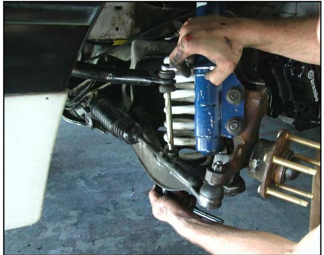
6. Loosen the tie-rod end nut but do not remove it.
