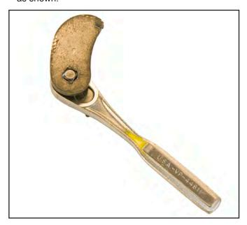
Fit the slotted end of the tool over the flange as shown. The flange can be bent by pushing down on the wrench. Reference the photo in the previous step to see where the tool needs to be used.
