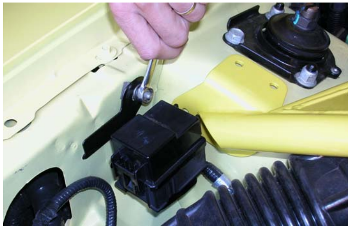
Vacuum Distribution Block Bracket (Driver's side rear of engine block)
