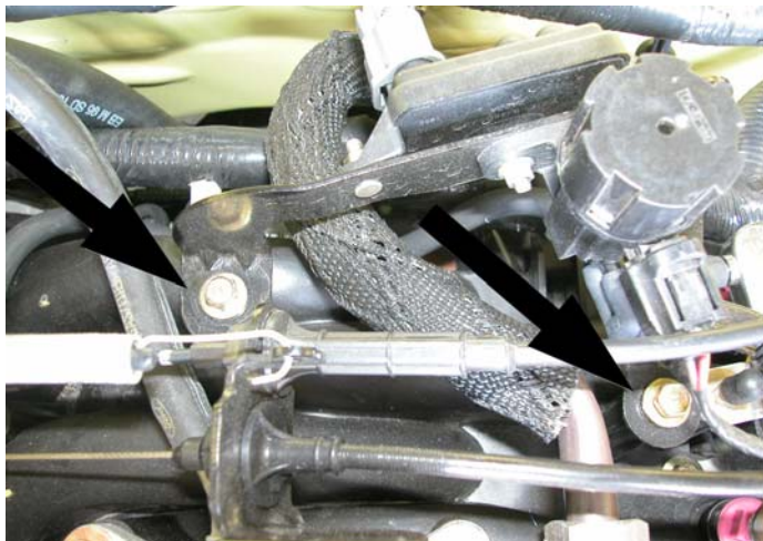
Vacuum Distribution Block Bracket (Driver's side rear of engine block)
