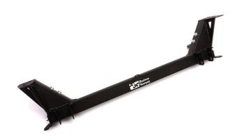
Maximum Motorsports' lightweight radiator core support for 2005-14 Mustangs is more than strong enough to support front swaybar loads. This unique, versatile product also features a swaybar mounting feature; allows mounting reinforcement braces between MM Core Support and the MM K-member; and makes it easy to mount a splitter or other accessories to dedicated tabs. Welded-steel construction and a corrosion-preventing, powdercoated finish complete the package.
