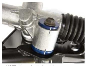
NOTE: It is easiest to install the spacers on one side of the steering rack at a time.
