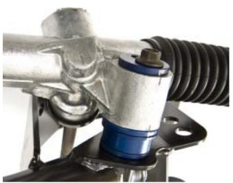
NOTE: If the rubber cover of the steering shaft input still rubs on the K-member, the black cover can be removed or trimmed.
